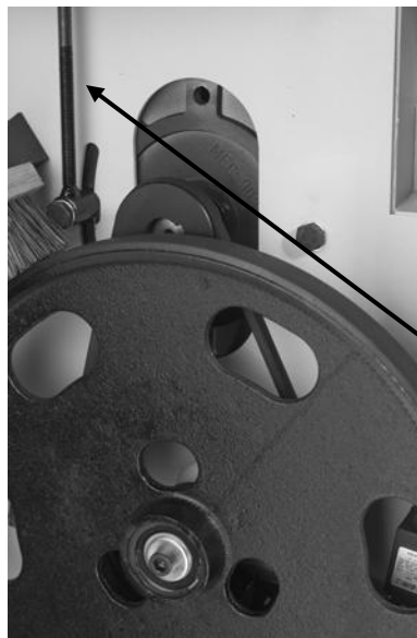
Belt tensioning bolt
